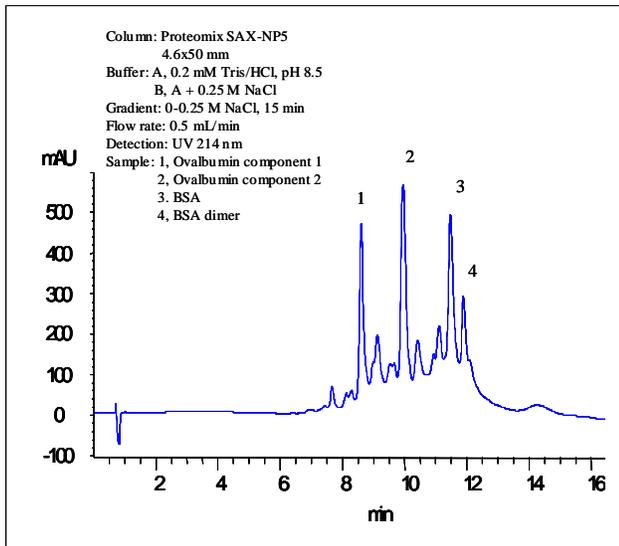
Figure 3. Elution profile of a mixture of ovalbumin and BSA by a *Proteomix* SAX-NP5 column.
