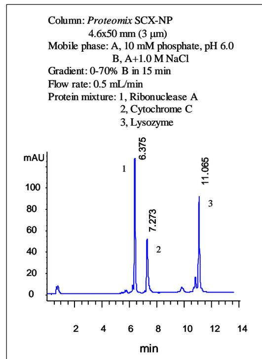
Figure 2. Separation of a protein mixture by a *Proteomix* SCX-NP3 column.
