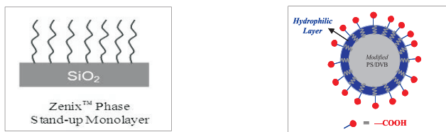
Figure 1. Phase structures for both the surface of Zenix™ SEC and Antibodix™ WCX.
