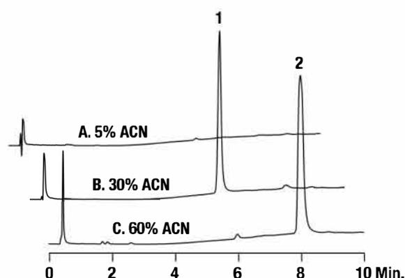
Column: Vydac<sup>®</sup> C4, 5 $\mu$ m, 50 x 4.6mm (Part No. 214TP5405)
