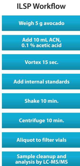
Figure 3: An example in-line sample preparation workflow for high-fat avocado samples.
