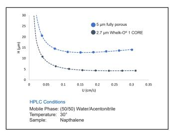
WHELK-0° 1 Core provides higher column efficiencies than similarly-sized fully porous particles, even at higher mobile phase linear velocities. H vs U curves compare performance of 2.7  $\mu m$  WHELK-0° 1 Core and 5  $\mu m$  fully porous WHELK-0° 1.
