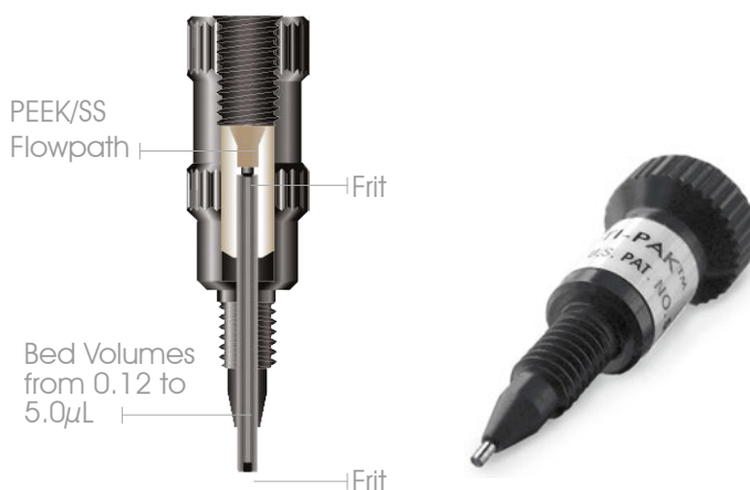
FLOATING STEM DESIGN FOR ZDV CONNECTION INTO ANY PORT
