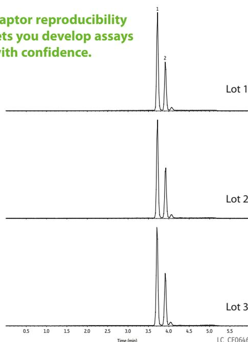
**Column:** Raptor FluoroPhenyl (cat.# 9319A1E); Dimensions: 100 mm x 3 mm ID, Particle Size: 2.7 µm; Temp.: 30 °C; **Sample:** Diluent: Water:methanol (50:50); Conc.: 25-50 ng/mL; Inj. Vol.: 5 µL; **Mobile Phase:** A: 0.1% Formic acid in water; B: Methanol; **Gradient (%B):** 0.00 min (75% B), 4.00 (85% B), 4.10 (100% B), 5.00 (100% B), 5.01 (75% B), 7.00 (75% B); **Flow:** 0.6 mL/min; **Detector:** MS/MS; Ion Mode: ESI+; Mode: MRM; **Instrument:** HPLC.
