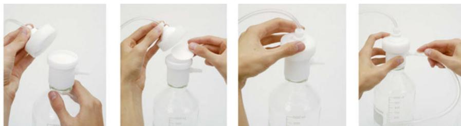
Unscrew and lift off top. Place membrane filter on top of grid. Reattach top. Connect vacuum line to side port.
