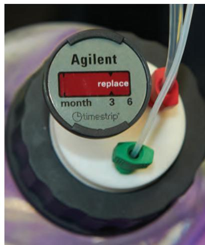
**Stay Safe caps** include a time strip that tells you when the venting valve needs to be replaced. We recommend changing the A-Line venting valve or the A-Line charcoal filter after six months of usage under the following conditions:
