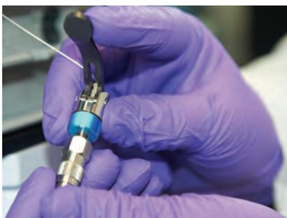
**As easy as closing a lever:** The proprietary Agilent design features a spring-loaded mechanism for zero dead volume and a sure, tight connection.
