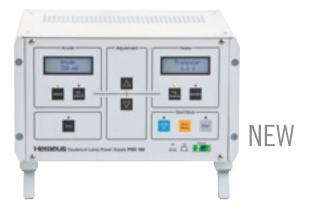
The PSD 186 R&D Deuterium Lamp Power Supply is the replacement for the high performance power supply PSD 181. A completely new design to incorporate state-of-the-art electronics, the PSD 186 is compatible with virtually all 30W Deuterium Lamps currently on the market.
