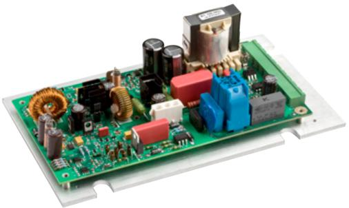
The PSD 184 Deuterium + TH Lamp Power Supply is a high performance, compact and highly reliable switching power supply. It is designed to operate on an 85–264 VAC input voltage. The supply has very low noise and drift characteristics and uses a novel ignition circuit (US patent No.5.530.319; EP No. 94 118 802.1) to ensure a soft and reliable arc ignition, even when the lamp is hot.
