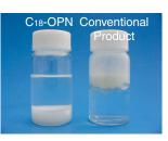
Packing materials in water Left : C18 OPN provides good resolution Right : Conventional product float up
