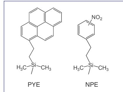
COSMOSIL PYE (Pyrenylethyl group bonded) and COSMOSIL NPE (Nitrophenylethyl group bonded) column show unique retention characteristics based on multiple separation modes such as hydrophobic, charge transfer and π-π interactions. These columns are recommended for the separation of structural isomers.
