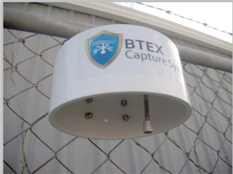
Figure 1. A BTEX Monitoring Tube (Camsco Part Number BTEX-T ) protected by tube shelter and Passive Sampling Cap (Camsco Part Number BTEX-S and DC60 , respectively)
