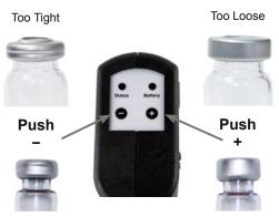
2. Step - Performe a crimp test before using your sample vials
