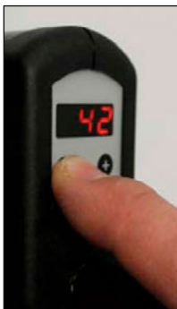
Figure 7. The numerical setting of the crimping tool sets a stop position that determines the amount of compression of the cap and is very accurate. There may be some drifting in the setting over
