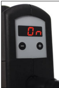
Figure 6. The display will show On momentarily and then enter operating mode.
