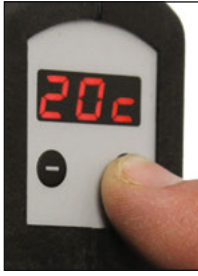
Figure 5. When the selection is complete, press and hold the go-button for 2 seconds to confirm the selection.
