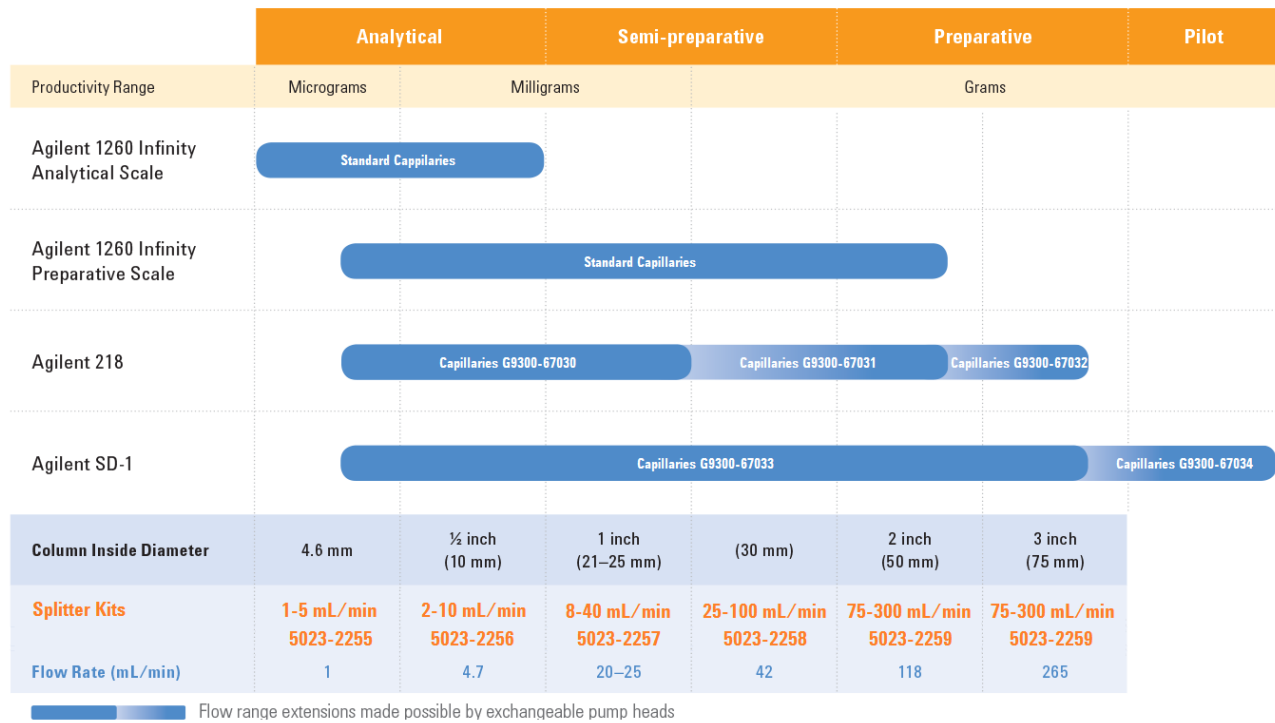
Figure 1 Splitter and capillary kits available for the different flow rate ranges and purification systems
