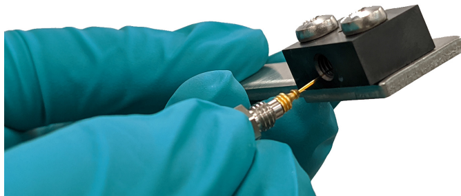
Figure 4. Thread the internal nut into the swaging wrench.
