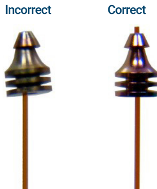
Figure 7. Incorrect and correct swaging symmetry.
