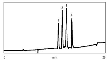
Figure 2. Peptide mixture on VariTide RPC 250 x 4.6 mm ID column at 0.5 mL/min, 40 °C. Gradient elution of 0-50% B in 20 minutes. Compounds: 1. Oxytocin, 2. Angiotensin II, 3. Angiotensin I, 4. Insulin.
