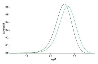
Figure 3. Overlaid molecular weight distributions of 2 nylon samples on 2 Agilent PL HFIPgel 9 µm columns.
