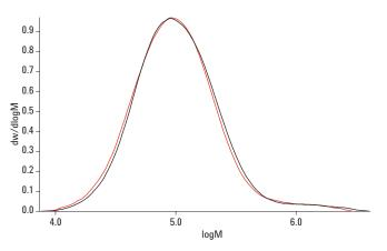
Figure 6. Overlaid molecular weight distributions of nylon samples on 2 Agilent PLgel 10  $\mu m$  MIXED-B columns with m-cresol as solvent.
