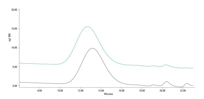
Figure 2. Raw data chromatogram of 2 nylon samples on a 2-column set of Agilent PL HFIPgel 9 µm columns with HFIP solvent.
