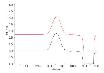
Figure 5. Raw data chromatogram of a sample of nylon on a 2-column set of Agilent PLgel 10  $\mu m$  MIXED-B columns with m-cresol.
