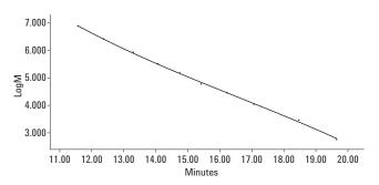
Figure 4. Calibrating the Agilent PLgel 10  $\mu m$  MIXED-B column using Agilent EasiCal PS-1 standards.
